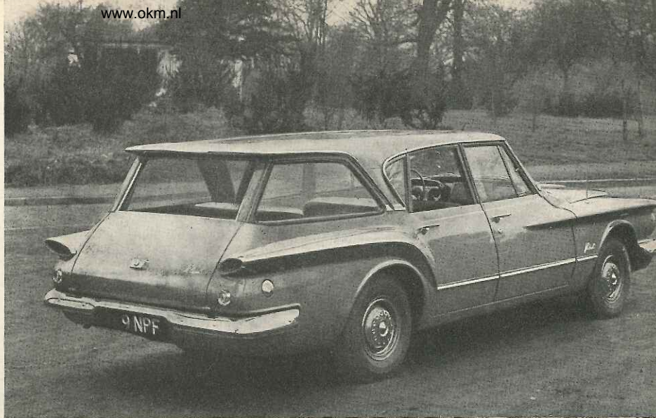
CURVED quarter windows and slim pillars provide a fine view backwards when the not-so-compact car is being reversed.
