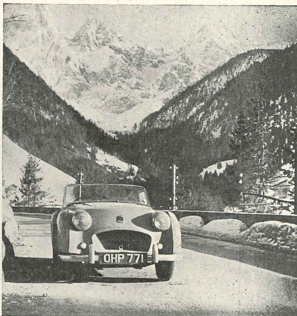
LOW FRONTAL AREA gives minimum air resistance but leaves useful internal roominess. High-mounted headlamps have a useful range but give a very limited sideways spread of light.
