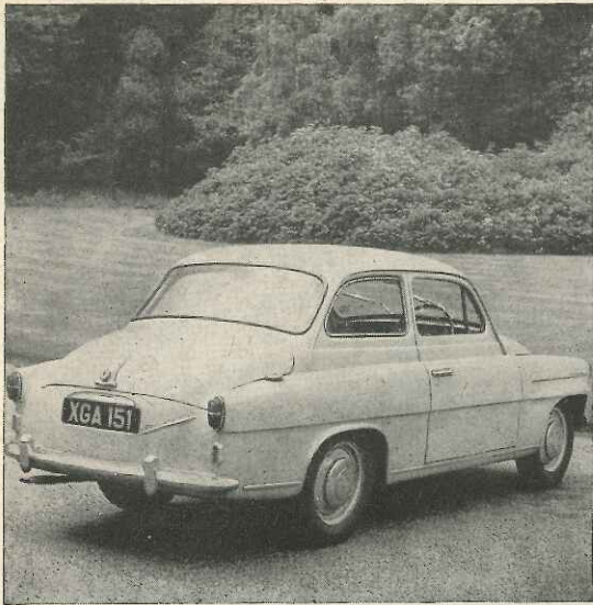
Some idea can be gained of the good fore and aft visibility provided by a quickly falling bonnet line and a very large rear window.
