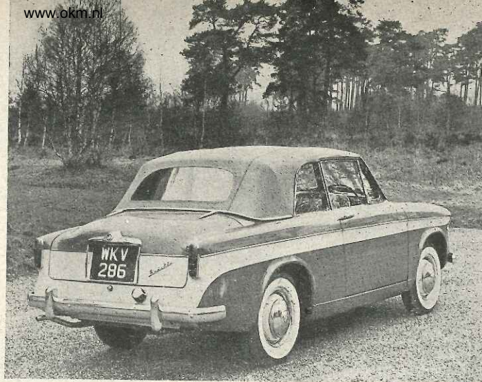
SPACE for luggage under the self-supporting boot lid remains ample despite the fabric bag into which the hood folds. The generous rear window is of clear flexible plastic.
