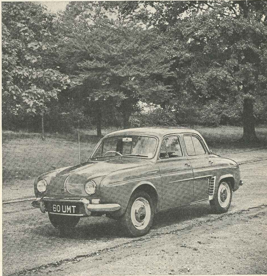
CONVENTIONAL in general proportions, but with its rear-mounted engine disclosed by cooling air intakes ahead of the rear wheels instead of at the front of the car, the Renault Dauphine is one of the best-looking small four-door saloons.
