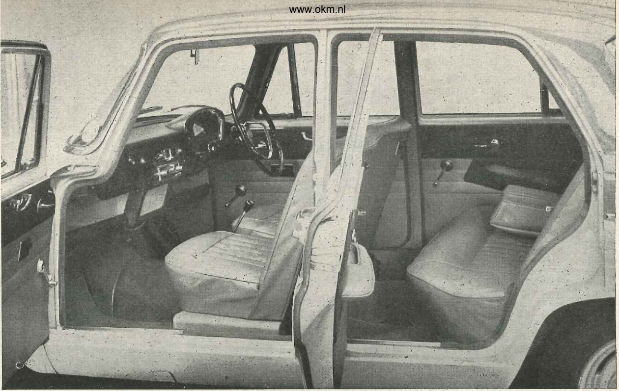
Big door openings make the four seats easy to enter. The interior is upholstered in leather, shod with carpet and decorated with polished walnut. The instrument panel and scuttle are finished in matt black.
