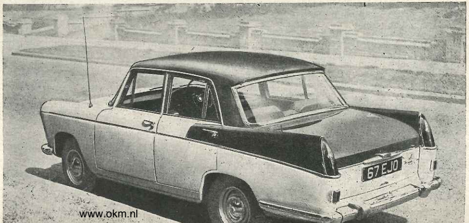
A prominent tail houses very large luggage capacity, with the spare wheel in a separate tray underneath and lockable petrol filler at the top.
