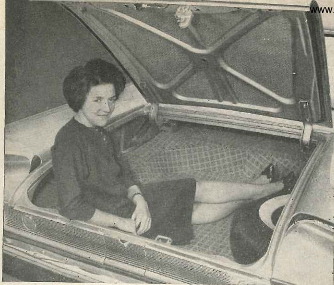
AREA of the luggage space provided in the large tail is evident from this photograph, the spare wheel and 8.00-14 tyre occupying a corner of the big locker.
