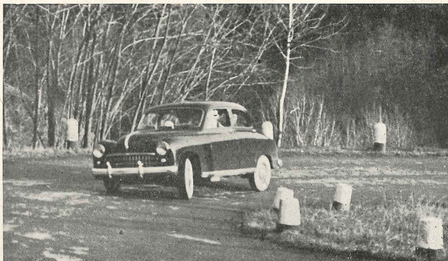
PERFORMANCE on hills in top gear is improved when a 1.9-litre compression-ignition engine is installed in the Fiat 1400, here seen cornering fast on a road through the Alpine foothills.
