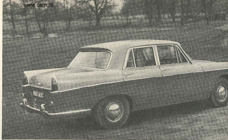
FINS of restrained size help a driver to park a large car accurately in confined spaces, without being a nuisance in other respects: stability in windy weather is good.
